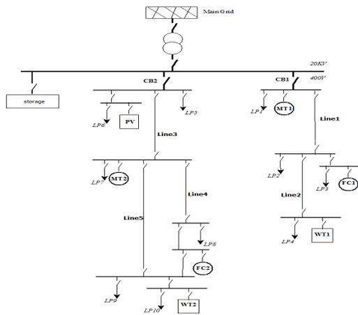
Fig.1.The sample microgrid
