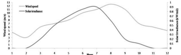
Fig.3.Forecasted wind speed and solar irradiance
