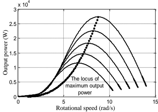
Fig.2. Output power versus rotational speed
