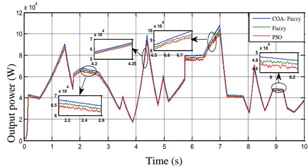
Fig.13. Simulation results in fast variations of the wind speed
