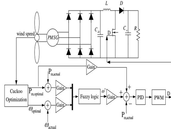
Fig.7. Completely schematic diagram of the proposed MPP tracker
