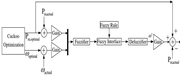
Fig.4. Configuration of the proposed MPP tracker
