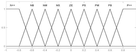
Fig.5. Input and output membership function of  $\Delta P_m$  and  $\omega^*$ , respectively
