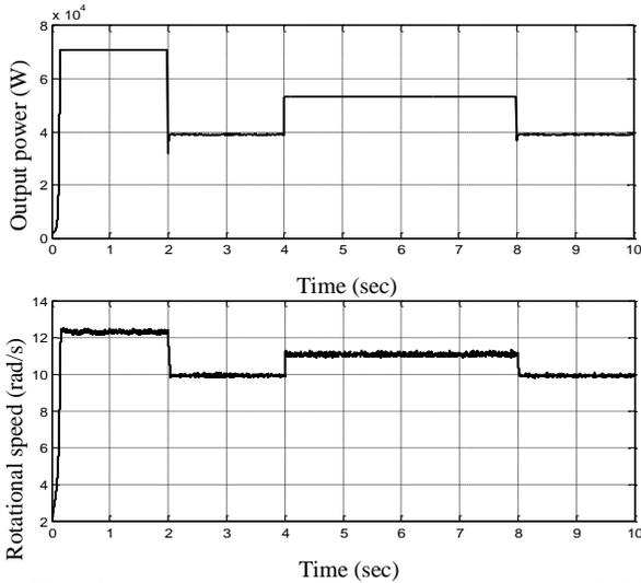
Fig.9. Output maximum power captured by the proposed MPP tracker and rotational speed calculated by cuckoo optimization algorithm while the wind speed is slowly changed
