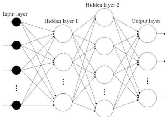
Fig.3. Schematic diagram of MLP structure.
