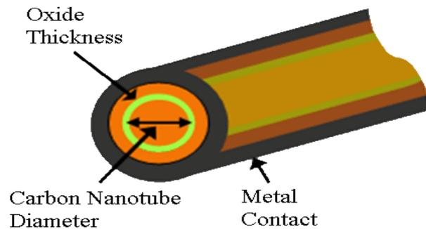
Fig.1. Optimized geometry assumed for CNTFETToy.
