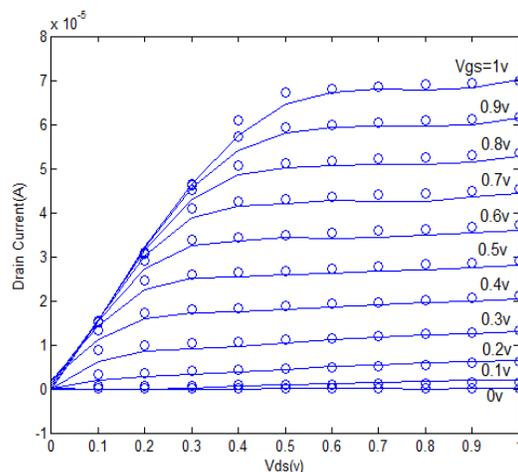
Fig.4. Current-voltage characteristics curve (Id-Vds) for CNTFET using CNTFETToy model (circle) and proposed ANN model (solid line).
