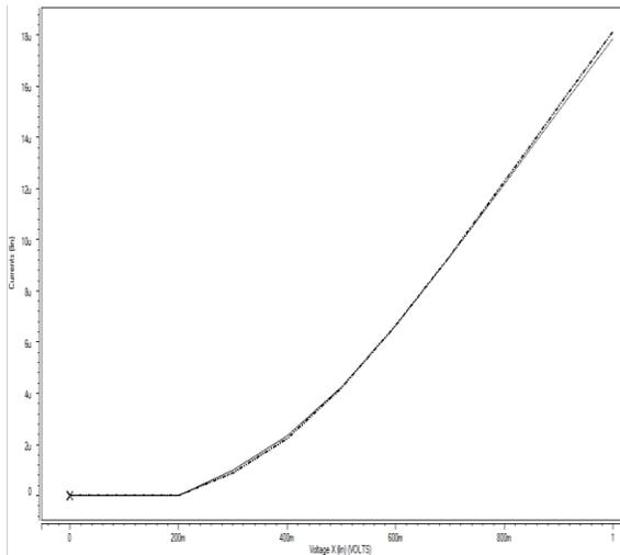
Fig.9. Output characteristic for ANN CNTFET current source ( $I-V$ ) solid line for ( $I_{ref}$ ) and dashed line for ( $i_{out}$ ).
