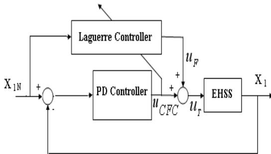
Fig.3. The EHSS velocity control with FEL method
