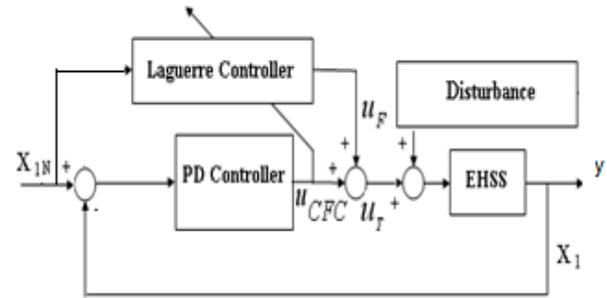
Fig. 7. Structure of controller in presence of Disturbance
