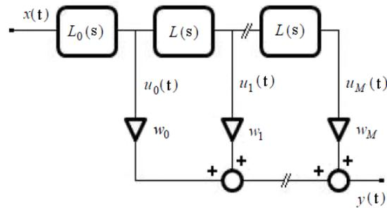
Fig.4. Basic diagram of Laguerre structure
