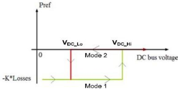
Fig. 4. Hysteresis controller operation
