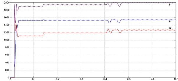
Fig. 8. Supplied P, Q, and S. PV generation is 75%.
