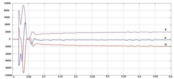
Fig. 10. Supplied P, Q, and S. PV generation is 0%.
