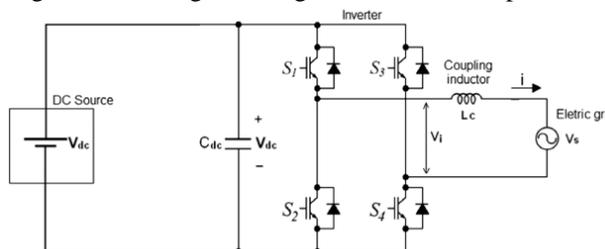
Fig. 2. General single-phase inverter system connected to the electrical power grid
