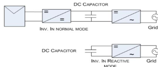
Fig. 3. Inverter switching to reactive mode
