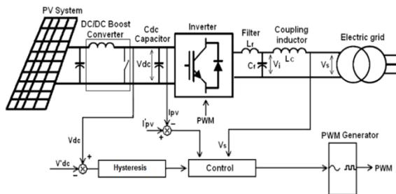
Fig. 5. Power system and control of the grid connected PV system
