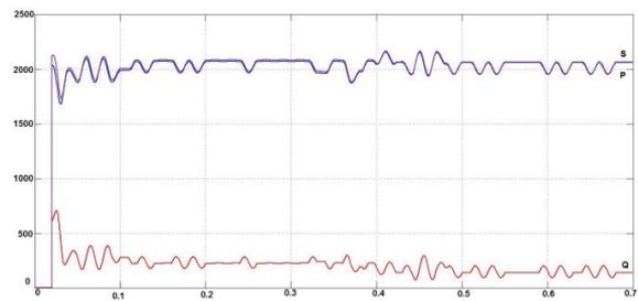
Fig. 9. Supplied P, Q, and S. PV generation is 100%.
