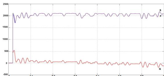
Fig. 13. Supplied P, Q, and S. PV generation is 100%.
