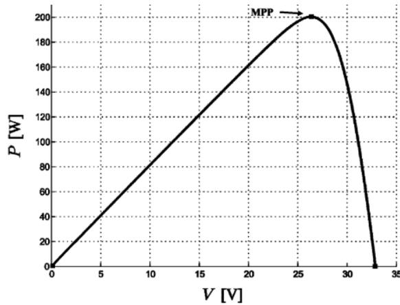
Fig. 1. V characteristics of a module under full solar irradiation [2]
