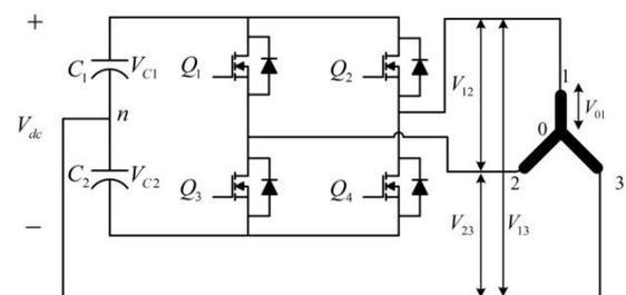
Fig. 2. B4 inverter configuration [12]
