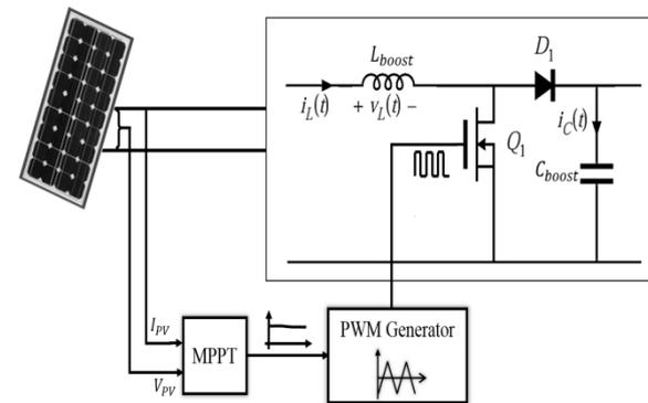
Fig. 4. Module integrated boost converter with MPPT and PWM control blocks.
