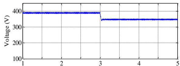
Fig. 8. Variation of the dc link voltage under the partial shading condition.
