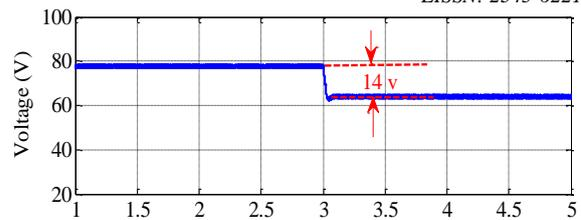
Fig. 7. Variation of the output voltage of the first Boost converter under the partial shading condition.
