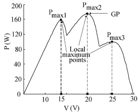
P—V characteristic of a module with bypass diodes in partial shading condition [4].
