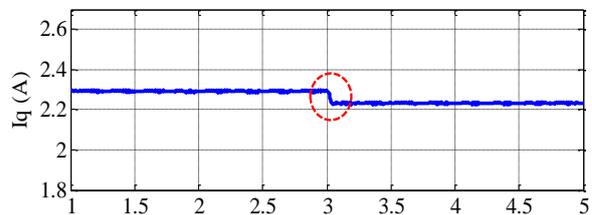
Fig. 9. Current of the q-axis (Iq) in Park Transformation.
