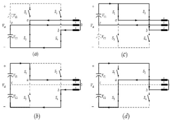
Fig. 5. Sub-operating modes of B4 inverter (a) mode I, (b) mode II, (c) mode III, and (d) mode IV [12].
