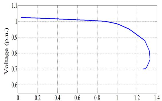
Fig. 3. Resulted PV curve of Bus 7 after G2 trip and adaptive load shedding.
