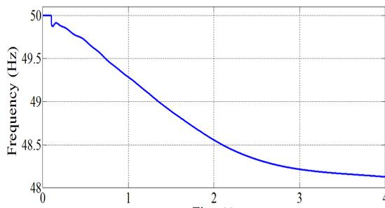
Fig. 4. System frequency for outage of the generator at bus 8 without UFLS.
