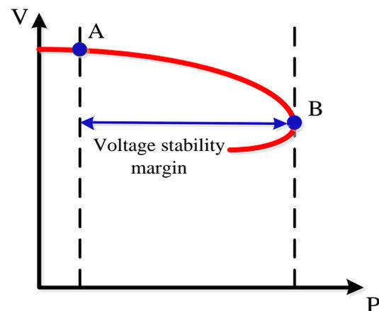
Fig. 1. A typical PV curve for a given condition.
