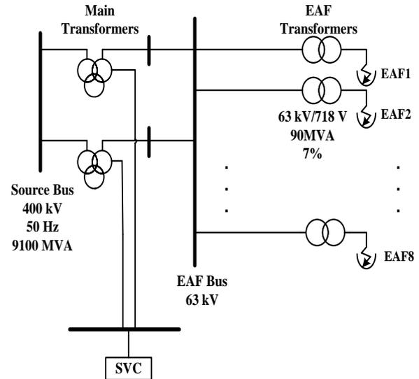
Fig. 3. Single line diagram of EAFs in Mobarakeh steel company system
