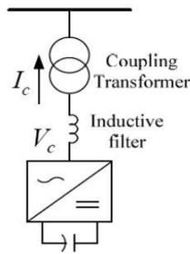
Fig. 2. Basic structure of STATCOM
