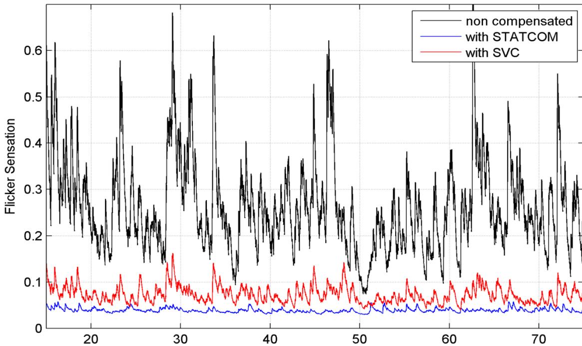
Fig. 6. Voltage flicker of Source bus (400 kV)
