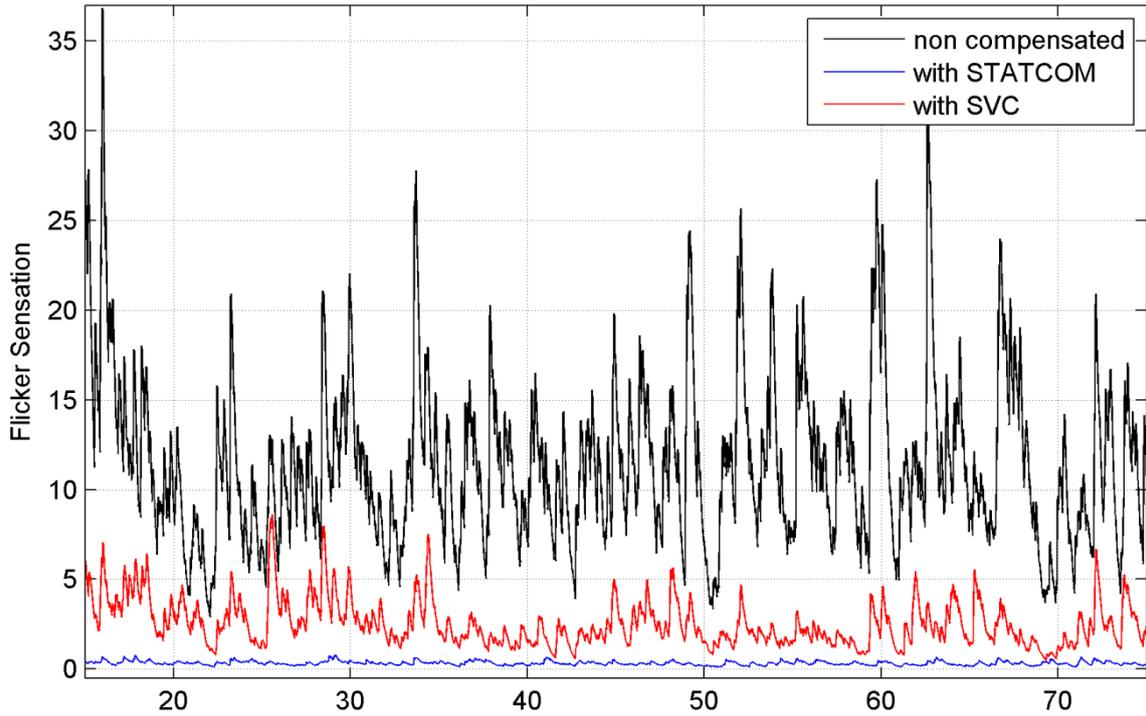
Fig. 5. Voltage flicker of EAF bus (63kV)
