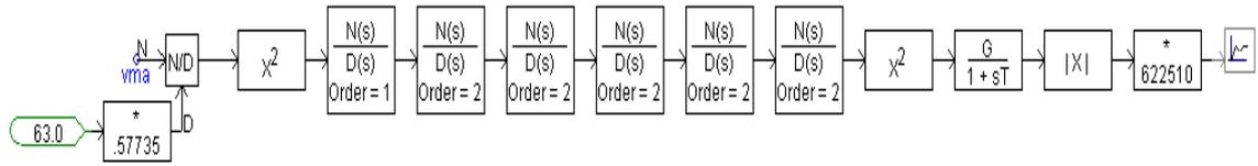
Fig. 4. Procedure of calculation the voltage flicker
