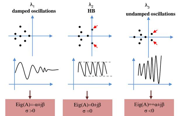
Fig. 1. Relation between the critical eigenvalues of dynamic algebraic Jacobian and power system oscillations
