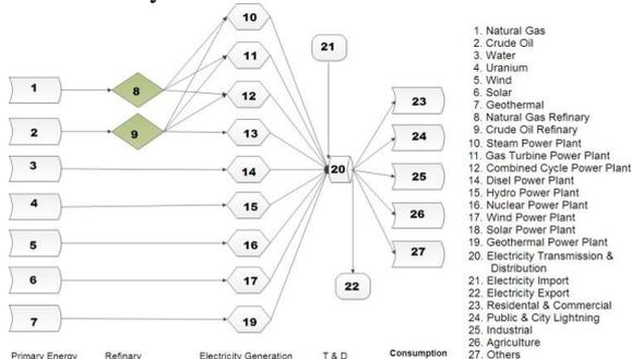
Fig. 1. Iranian Electrical Energy Flow as a Reference Energy System (RES) [2]
