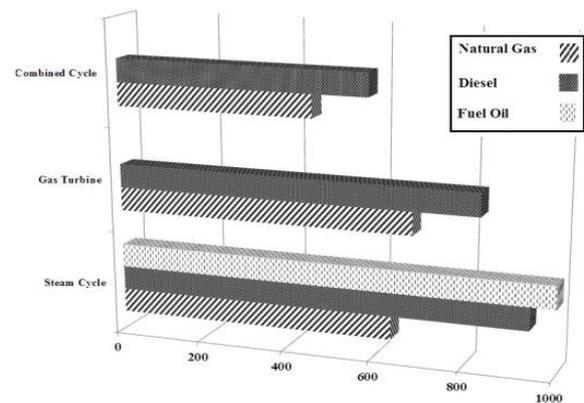
Fig. 3. CO<sub>2</sub> Emission from Iranian Thermal Power Plants (gram/kw-h) [2]
