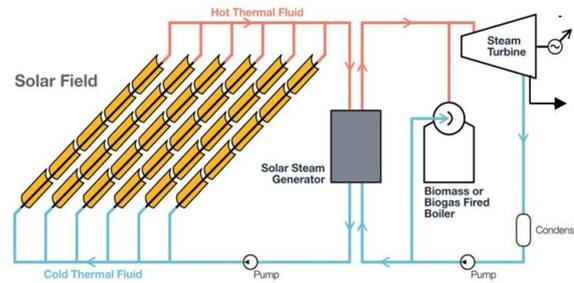
Fig. 3. Diagram of Biomass Solar Hybrid
