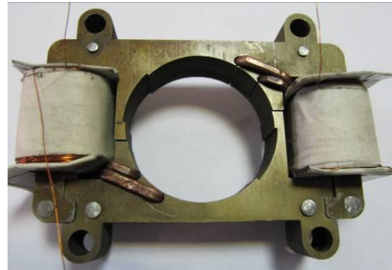
Fig. 7. Stator and its windings during the assembly process
