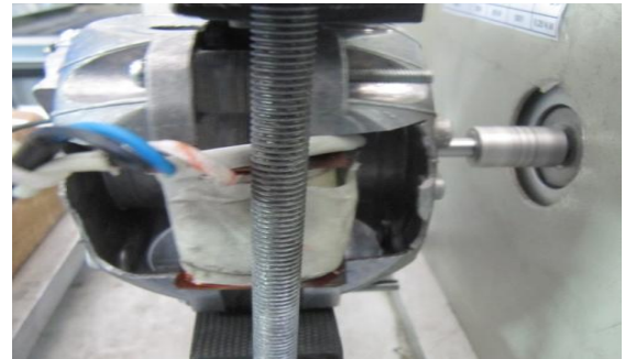
Fig. 9. Dynamometer test of the optimum restructured SPIM
