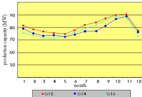
Fig. 1. Changes in production capacity gas power plant units in Fars Power Plant
