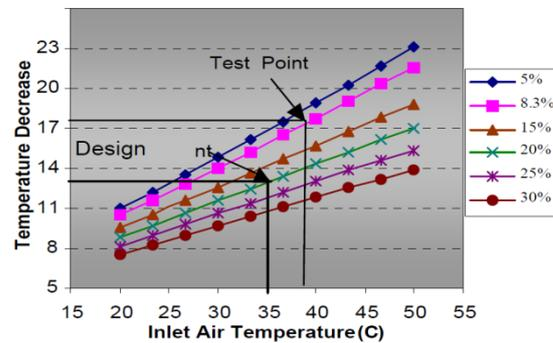
Fig. 8. Reduction of compressor inlet air temperature by Media evaporative cooler in different climatic conditions
