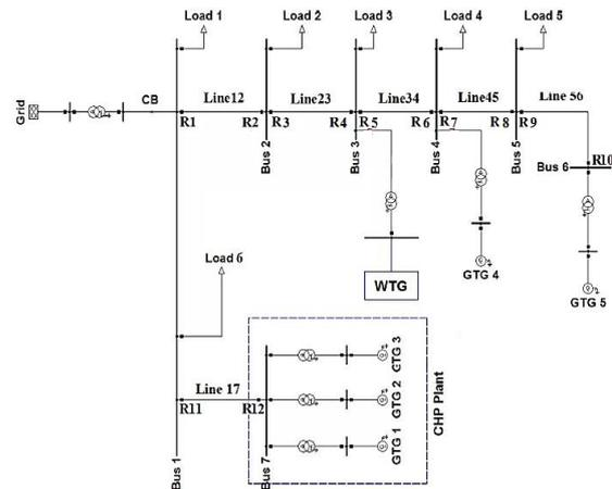
Fig. 3. Test distribution system [23].
