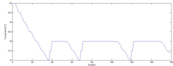
Fig. 8. Room temperature for set point =18°C
