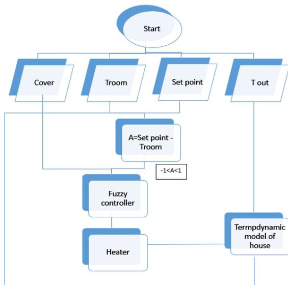
Fig. 1. Heating Control Algorithm
