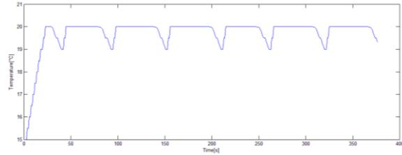
Fig. 7. Room temperature for set point =20 °C
