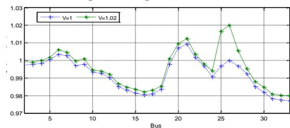
Voltage profile when DG<sub>1</sub> operates in the PV mode
