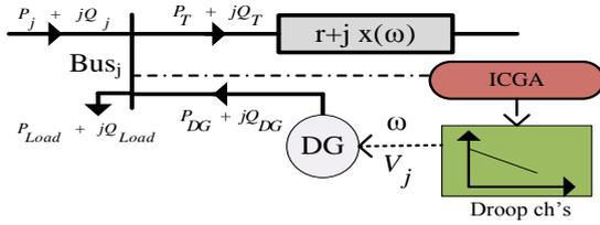
Injected power of DG to bus j based on droop
