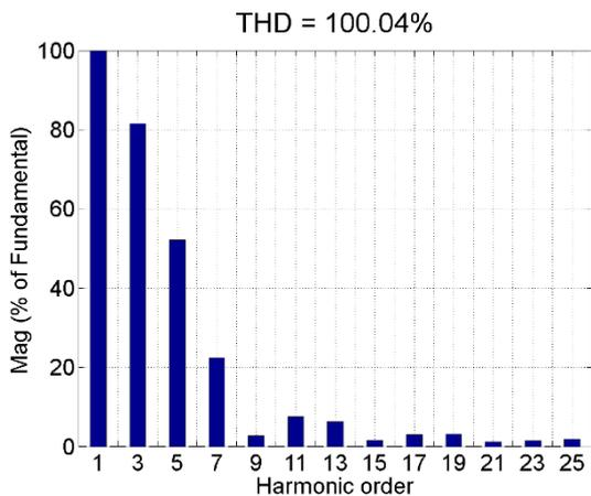
Fig. 5. Harmonic spectrum of the load current.
