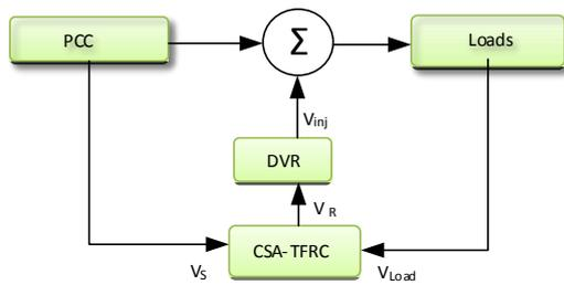
Fig.2 Proposed CSA-TFRC based DVR system
