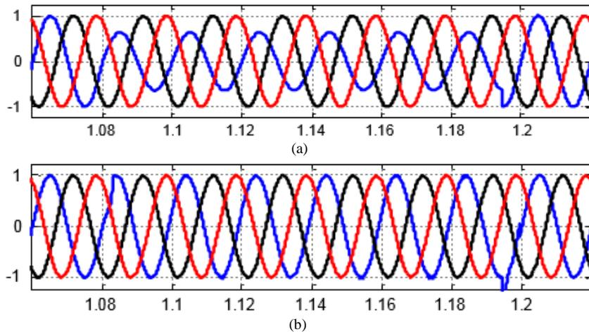
Fig.4 The p.u. voltages; (a) PCC voltage, (b) load voltage
