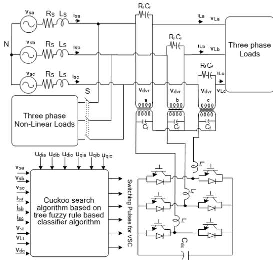
Fig.1 Single line diagram of DVR
