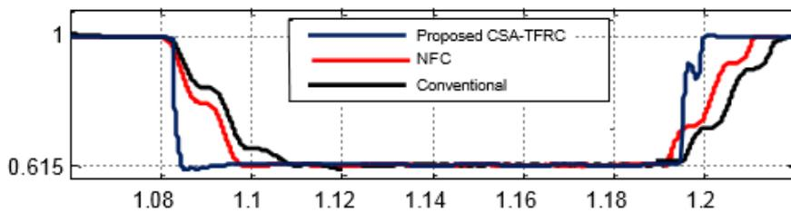
Fig.6 Estimation of voltage sag for phase A of PCC
