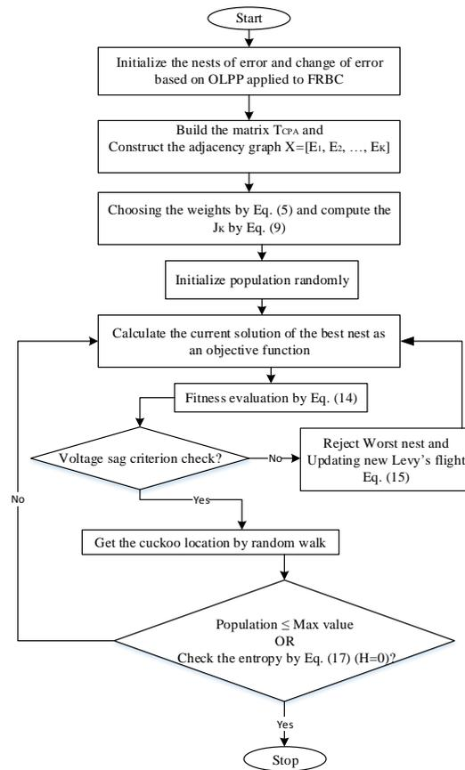
Fig.3 Proposed CSA-TFRC flowchart
