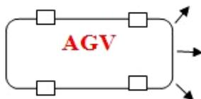
Fig. 1. Lidar Sensor arrangement
