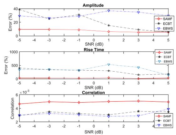
Fig. 6. Calculated factors for comparing denoising methods for the noisy PD signal 3 and Amplitude 50 mA
