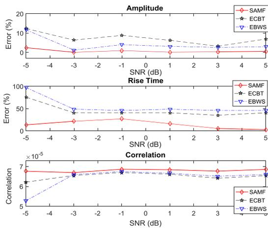
Fig. 5. Calculated factors for comparing denoising methods for the noisy PD signal 1 and Amplitude 10 mA
