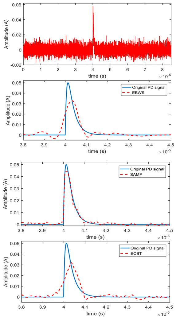
Fig. 7. Results of noise reduction for the noisy PD signal 3, Amplitude 50 mA and SNR= -5 dB
