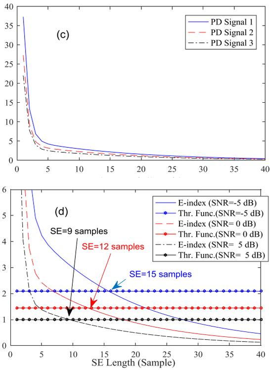
Fig. 3. a) The calculated  $e_j$  for the noisy PD signal and fitted curve (E-index) b) The E-indexes for three different noise levels c) The E-indexes calculation for three different PD signals d) The calculated thresholds and the selected SE length for denoising
