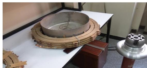
Fig. 4. Air-core laboratory winding
