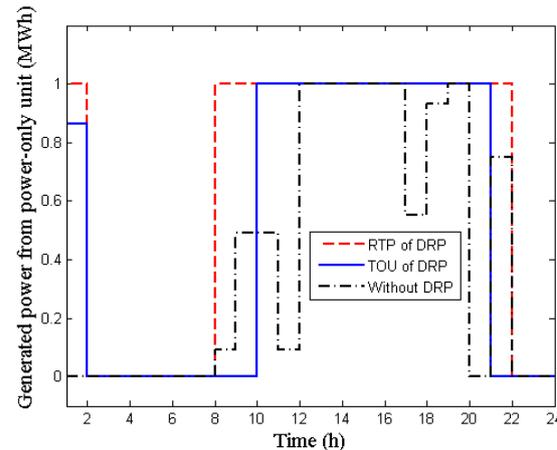
Fig. 5. Generated power by the power-only unit
