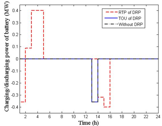
Fig. 7. Charging/discharging state of the battery storage system
