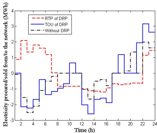
Fig. 2. Exchanged power with the MG and upstream grid
