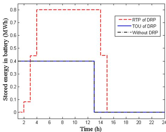
Fig. 6. Stored energy in the battery storage system
