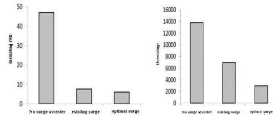
Fig. 10. Insulating risk (a) and maximum overvoltage (b) diagram in three modes: without surge arrester, with existing surge arrester and optimal surge arrester.
