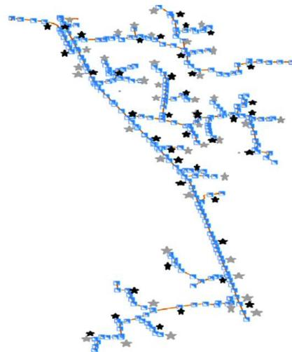
Fig. 9. Positioning the existing surge arrester and optimal arrester
