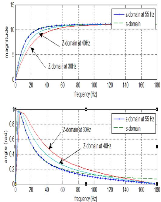
Fig. 6. Frequency response, effect of sampling frequency on the frequency response of the digital PSS
