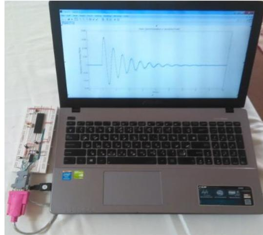
Fig. 11. The microcontroller based digital PSS hardware with MATLAB Simulink interface
