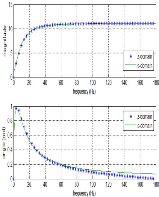
Fig. 7. Frequency response, comparison between the frequency response of the designed digital PSS and the response of the continues domain PSS
