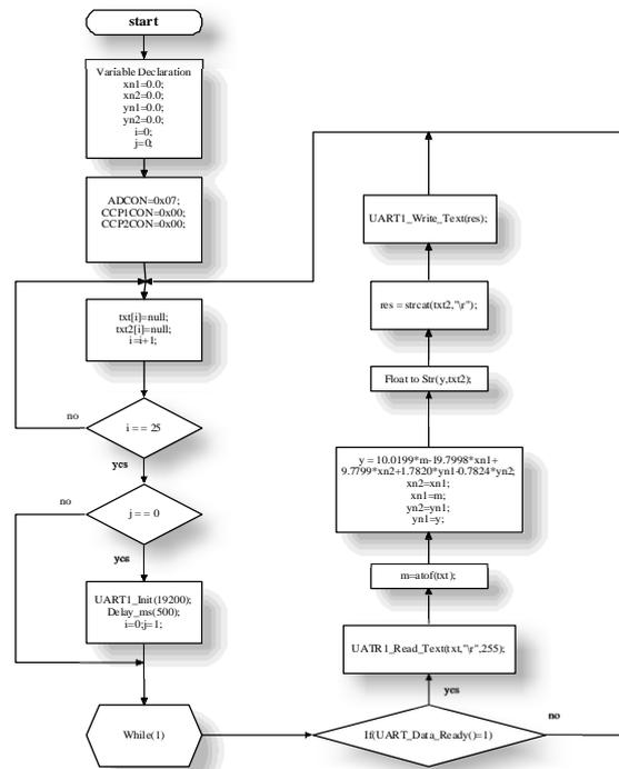
Fig. 8. Microcontroller C-code flowchart
