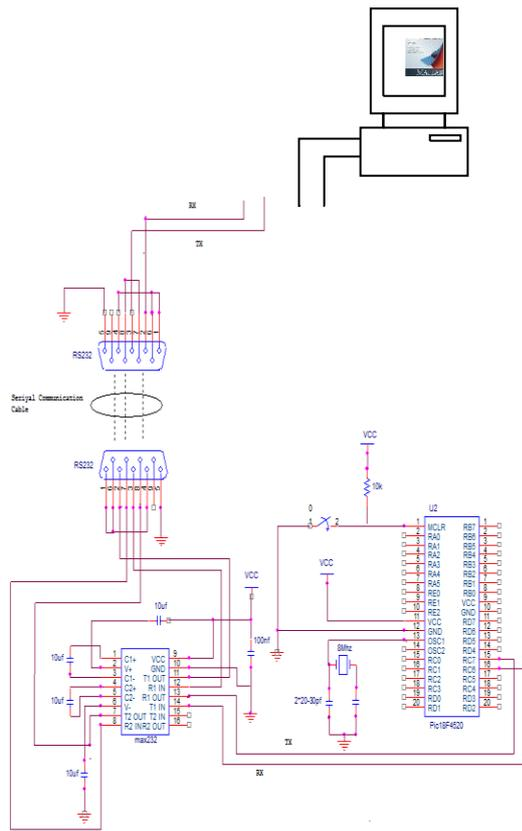
Fig. 9. MATLAB and PIC18F4520 microcontroller interfacing circuit
