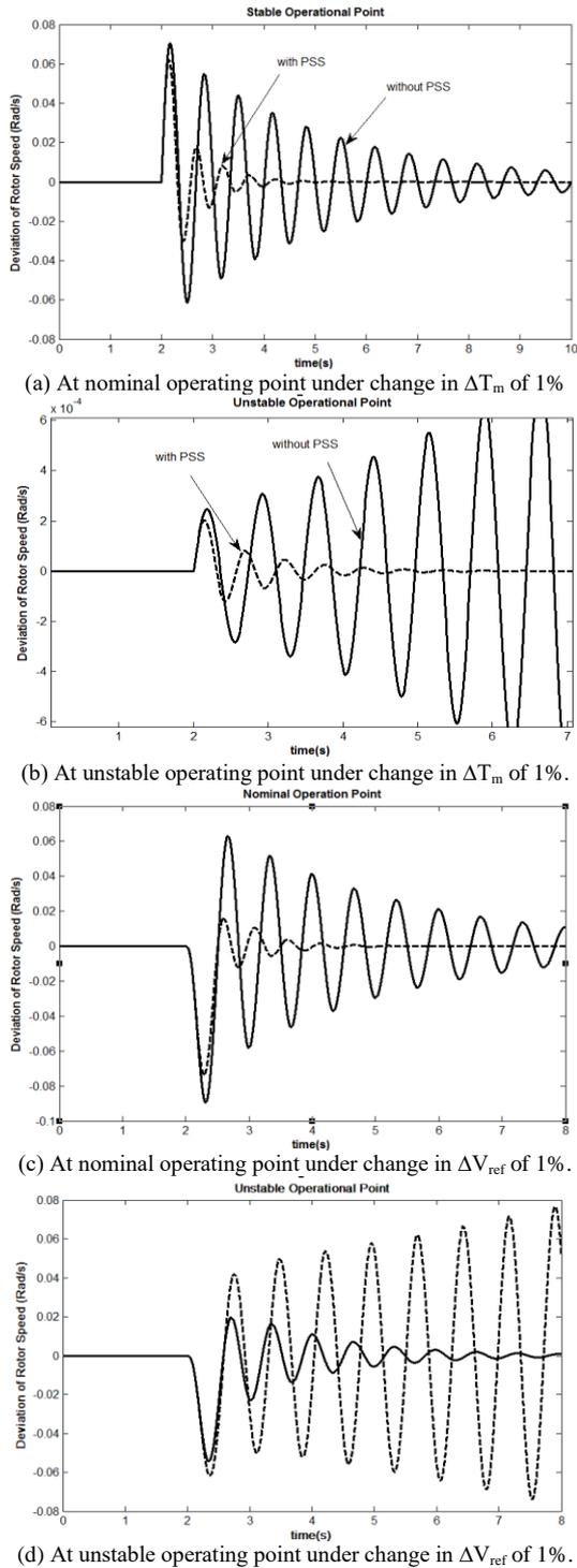
Fig. 5. Rotor speed deviation response with and without PSS
