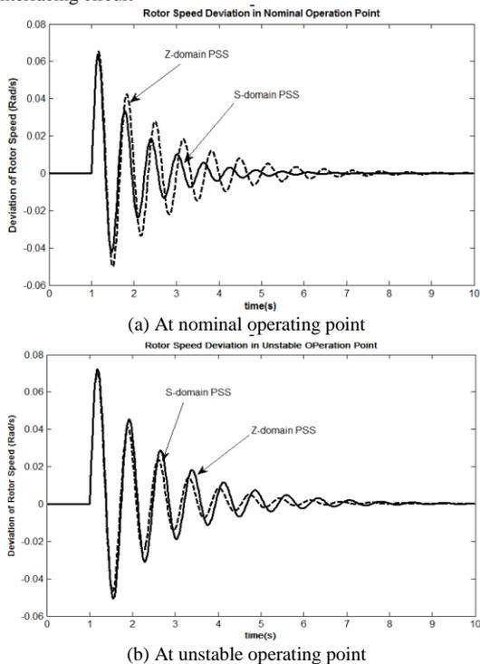
Fig. 10. Rotor speed deviation response comparison of digital PSS and continuous domain PSS under change in  $\Delta T_m$  of 1%.
