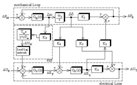
Fig. 1. Single-machine infinite-bus (Block diagram of SMIB system with PSS)
