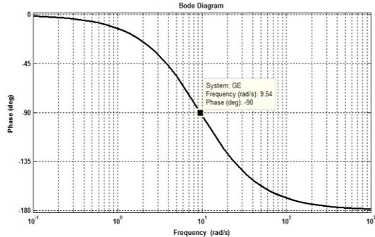
(b) Phase diagram of transfer function  $G_E(s)$
