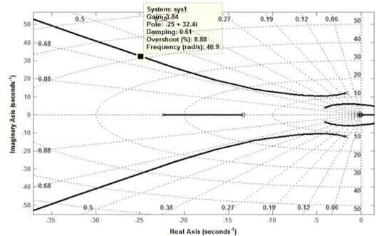
(c) Showing gain compensation in accordance with the optimum damping
