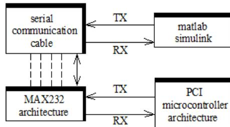
Fig. 3. Block diagram of MATLAB and microcontroller interface
