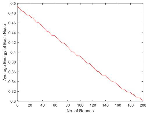
Fig. 5. Average residual energy of sensor nodes
