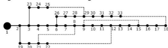
Fig. 2. Single line diagram of 33 bus system before reconfiguration
